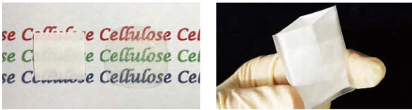
Thermoforming of thermoplastic cellulose (Left: before heat pressing, Right: after heat pressing) Heat sealability of thermoplastic cellulose
