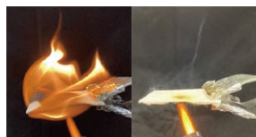
Combustion test of flame-retardant cellulose (Left: pulp, Right: flame-retardant cellulose)
