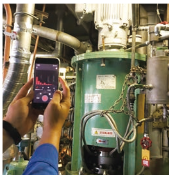
Using a smartphone (existing infrastructure) to gather noise data on equipment being monitored by sensors
